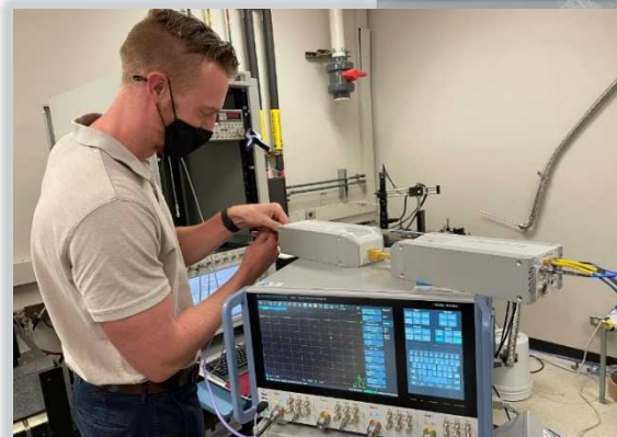
The R&S ZNA connected to R&S ZC170 frequency extenders allows S-parameter measurements in the D-band. (Image: Rohde & Schwarz)
